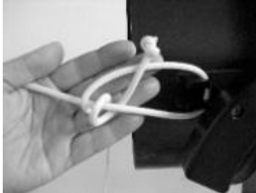
Rope fastening to the left handle
